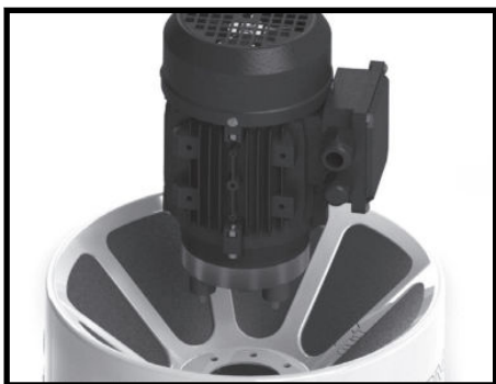
Step 13. Re-fit motor to top of case.
