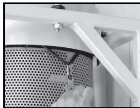
Step 3. Remove old seal.
