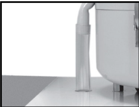
Step 4. Fit oil return tube and position tube to drain oil back to machine enclosure, sump or collection vessel.
