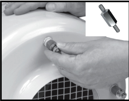
Step 1. Fit four case studs with the notched edge facing towards the Fil-termist unit (supplied with unit).
