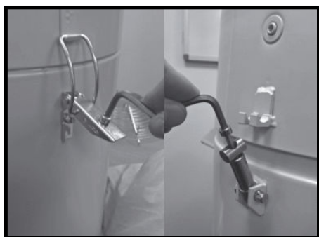
Step 1. Undo safety latch and clips.
