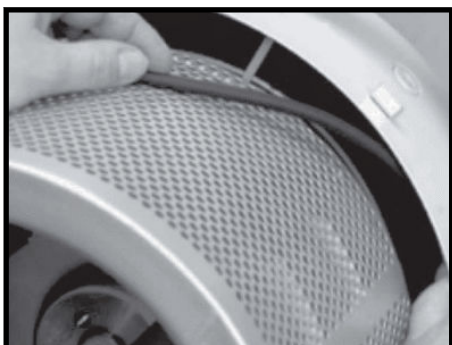
Step 16. Fit new seal.
