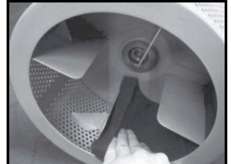
Step 6. Fit new drum pads.
