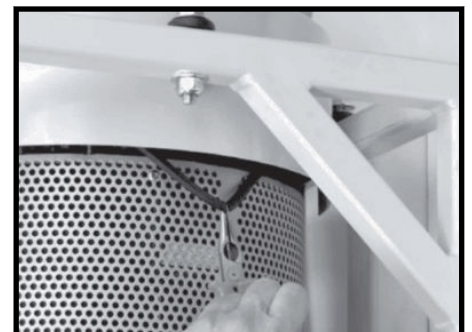
Step 3. Remove old seal.
