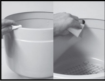
Step 4. Clean areas where top and bottom of case join and clean drain hole.
