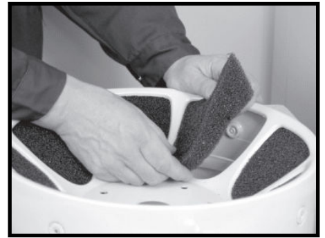
Step 12. Remove old silencer and fit new silencer.
